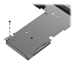
Removing the ExpressCard Assembly Screws
